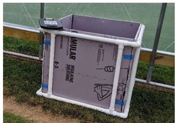
Figure 1. Water box used to contain 0.5 in. of water within the center of a plot.
